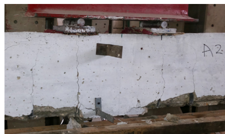
(b) Rupture of GFRP reinforcement bars
