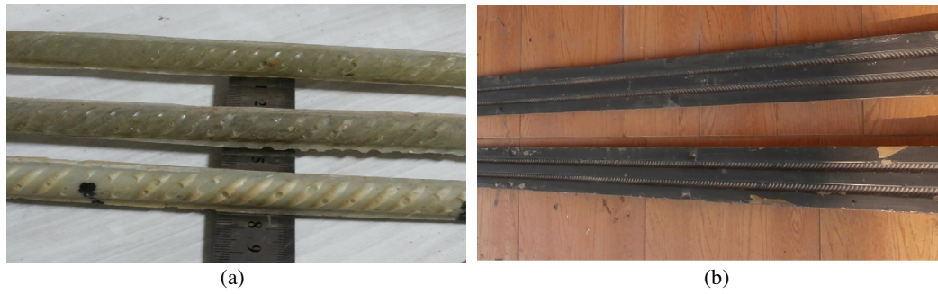
Fig. 1. Manufactured GFRP bars. (a) Ribbed 12 mm bars with Crescent shaped lugs (b) double sets of plastic mold.
